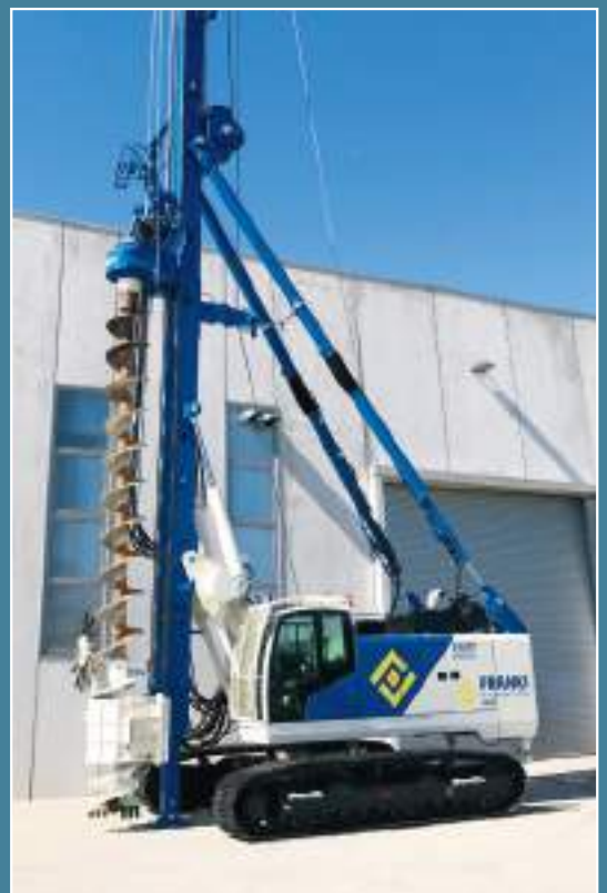
FRANCE E6050 LM - CFA240 CFA Piles.
