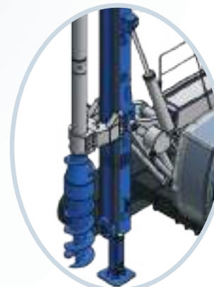
SP Soil Displacement
