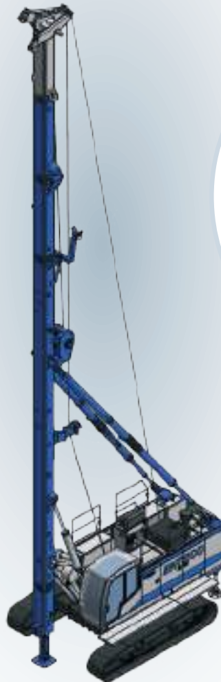
DTHR DTH piles with Tilting Rotary
