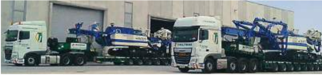
FRANCE E6050 LM – CFA240 CFA Piles.
