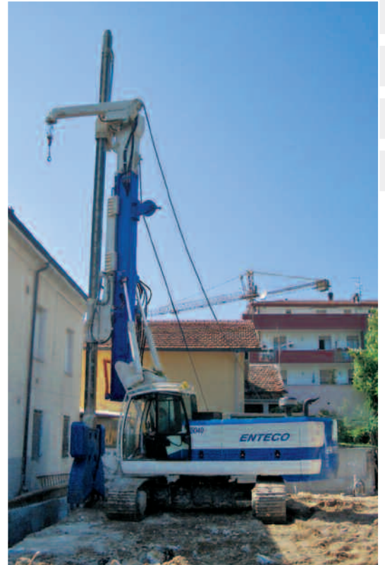
Rimini (Italy): E6040-HGM20. Diaphragm-walls 300 mm wide.
