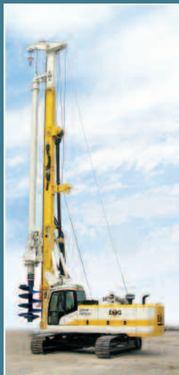
SPAGNA E6040M. con kit pali trivellati ed elica continua. Spain: E6040M. Dual-use rig: equipped with bored-piles and CFA attachments.
